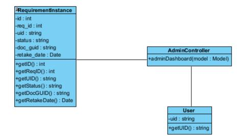
As with the student dashboard, the Java classes and methods associated with the admin dashboard are also fairly simple. We use the same MVC "magic" here as we do with the student dashboard, so most of the work of displaying the information is done programmatically in the HTML.
